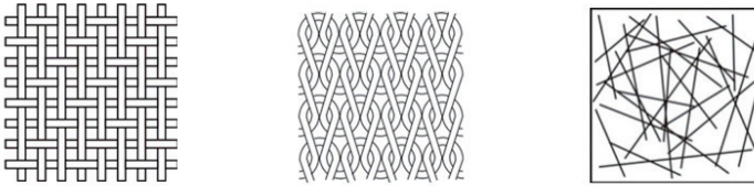
Figure 5. 2-D schematic presentations of woven-, knitted-, and nonwoven (made from staple fibres) fabrics
